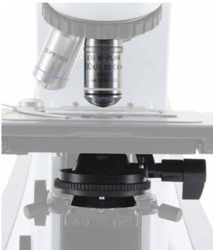
Brightfield: N.A. 0.2/0.9, swing-out, sliding-in and with centering system
