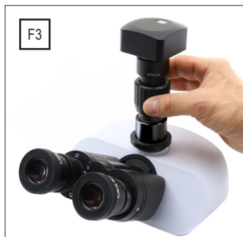
F1 / F2 / F3) While observing the image on the screen/monitor, adjust the focus by turning the knurled knob on the C-mount adapter
