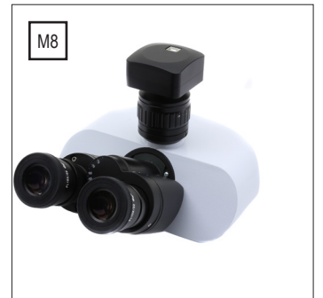
M7 / M8) Install the previously assembled C-mount + camera on the trinocular head
