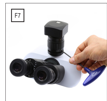
F7) Tighten the clamping knob on the 1x C-mount adapter
