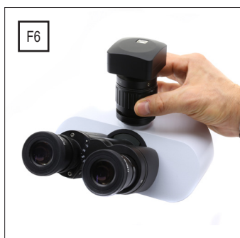
F6) While observing the image on the screen/monitor, adjust the focus by turning the knurled knob on the C-mount adapter
