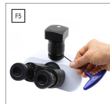
F4 / F5) Loose the clamping knob of the 1x C-mount adapter
