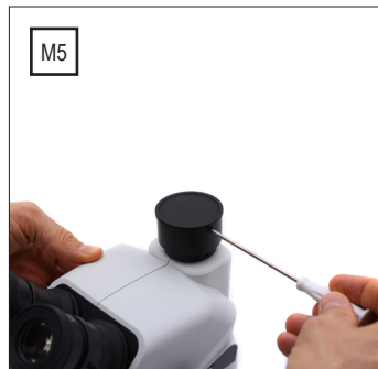
M5) Loose the clamping screw
