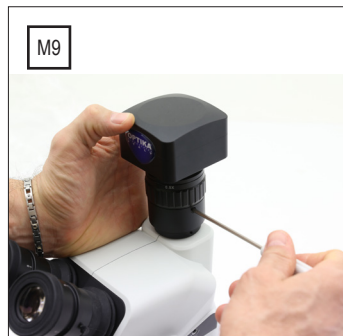
M9) Tighten the clamping screw firmly
