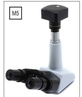
M5) Connect the C-mount projection lens on the trinocular port
