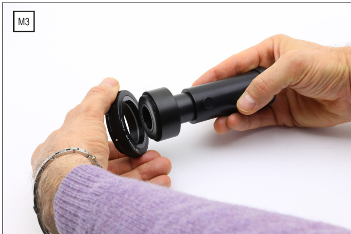
M3) Screw the Reflex adapter to the "T2" ring (provided with the Reflex camera or from its manufacturer)
