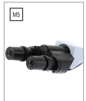
M5) Remove an eyepiece
