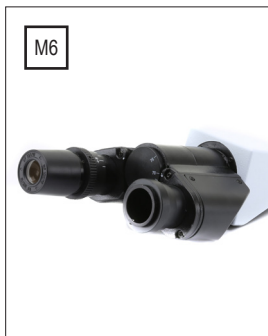
M6) Connect the C-mount projection lens where the eyepiece has been removed
