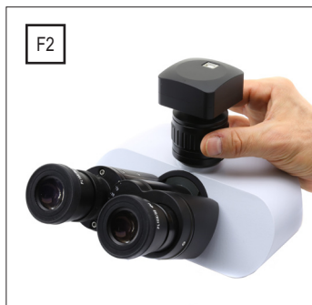
F1 / F2 / F3) While observing the image on the screen/monitor, adjust the focus by turning the knurled knob on the C-mount adapter
