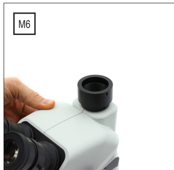
M6) Remove trinocular head's dust cover
