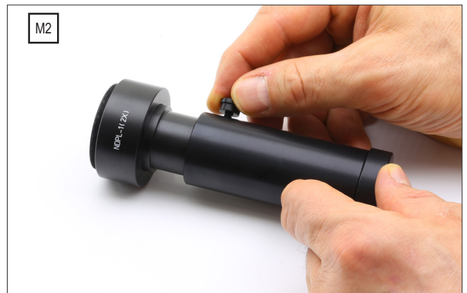
M2) Clamp the bottom part of the Reflex adapter with the universal adapter
