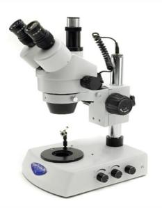
Gemological trinocular stereozoom microscope, 7x...45x, pillar stand, transmitted & incident light
