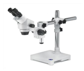
Binocular stereozoom microscope, 7x...45x, overhanging stand
