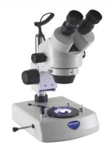
Gemological binocular stereozoom microscope, 7x...45x, pillar stand, transmitted & incident light
